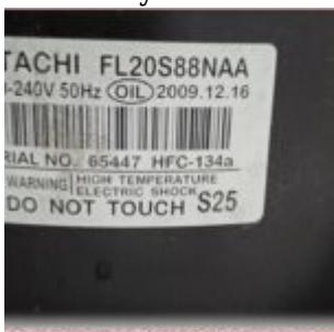
The HITACHI FL20S88NAA 0.75 HP hermetic scroll compressor delivers 256W cooling capacity at 50Hz, utilizing HFC-134a refrigerant for household refrigerator-freezer applications. This LBP-classified unit operates reliably at 220-240V with RSIR starting method, integrated into Sharp's SJ-PT73R-HS3 model offering 662-liter gross capacity with Hybrid Cooling System and Plasmacluster technology.
