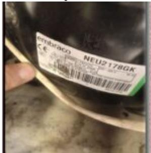
The Embraco NEU2178GK is the definitive choice for 1 HP commercial freezing applications. Featuring a robust CSR motor and 16.8cc displacement, this R404A compressor delivers high starting torque for demanding environments. This guide details the electrical requirements, installation tips, and how it compares to Secop and Tecumseh alternatives.
