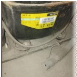
Secop SC21G is a high-performance hermetic reciprocating compressor designed for commercial refrigeration and freezing applications using R134a refrigerant. This guide covers detailed specifications, technical parameters, and installation requirements for 220-240V/50Hz systems at up to 1.3 amperes.
