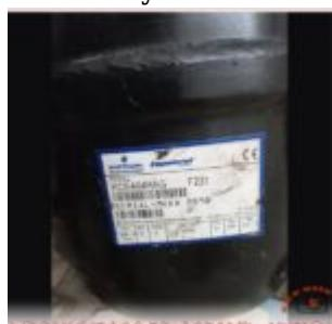
Copeland KCE444HAG Compressor, 3/8 Hp, R134a, 230V 50Hz - Technical Specs and Water Cooler Applications
