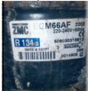
The ZMC EGM66AF is a high-reliability 1/6 HP compressor designed for Low Back Pressure (LBP) applications in domestic refrigerators ranging from 10 to 12 feet. Utilizing R134a refrigerant and a 6.66cc displacement, this unit features durable copper windings and an RSIR motor, making it a preferred choice for technicians seeking longevity and efficiency.
