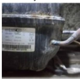
The Huayi HYE55YL63 and ZMC EGM60AF are two industry-standard 1/5 HP compressors used in domestic refrigerators. While both utilize R134a refrigerant, they differ in displacement and oil capacity. This technical review compares their performance curves and cooling capacities to help technicians select the ideal replacement for Kiriazi and other 14-foot refrigerators.
