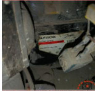
**Mbsmpro.com, Compressor, Danfoss, SLV15CNK, 15.28 cm<sup>3</sup>, LBP, Freezing, R290, Variable Speed, 220-240V 50/60Hz, Inverter, -40°C to -10°C**
