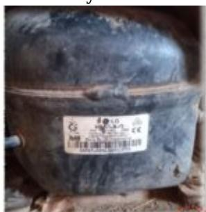
The LG MA57LBJG is a high-performance 1/6 HP compressor designed for R134a refrigerant in Low Back Pressure (LBP) applications. Ideal for domestic freezers, it delivers 160W of cooling capacity at -23.3°C. This guide provides comprehensive technical data, winding details, and a full cross-reference list for professional refrigeration technicians and engineers.
