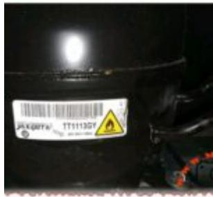
The Jaxipera TT1113GY is a high-performance hermetic compressor engineered for Low Back Pressure applications using R600a (Isobutane). Featuring a 11.3 cm<sup>3</sup> displacement and a cooling capacity of 183 Watts, it represents the gold standard for modern energy-efficient refrigeration, offering exceptional reliability and reduced acoustic emissions in the domestic market.
