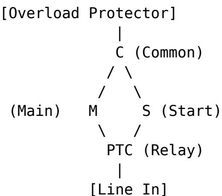
*(This schematic represents the typical PTC/RSIR wiring for the TT1113GY without a run capacitor.)*
