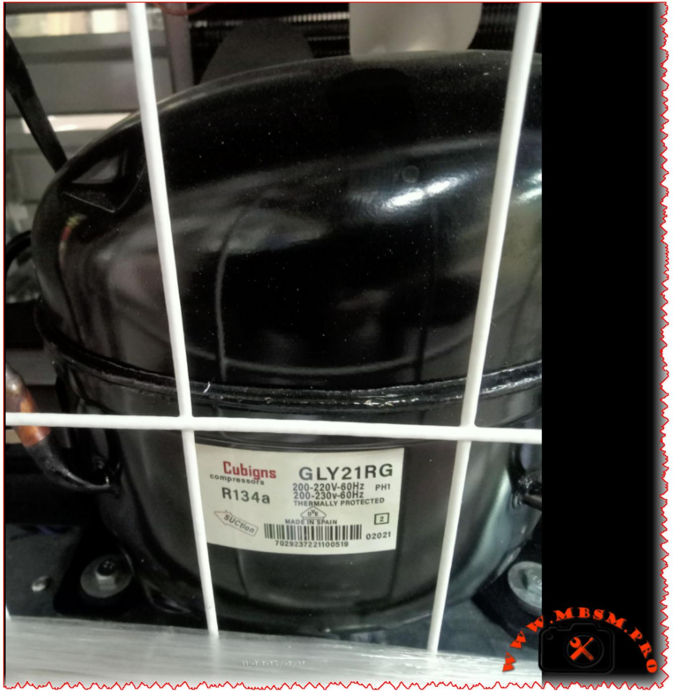
Cubigel GLY21RG R134a 5/8 HP Commercial Compressor Specifications and Replacement Guide
