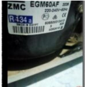
**Mbsmpro, Compressor, EGM60AF, 1/6 hp, ZMC, Cooling, R134a, 155 W, 1.1 A, 1Ph 220-240V 50Hz, LBP, RSIR, -35°C to -10°C, Cooling and Freezing**
