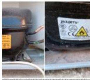
Based on the technical specifications of both compressors, it is **not recommended** to replace the burnt-out compressor (Jaxipera N1113Y) with the second one (ACC HTK70AA).
