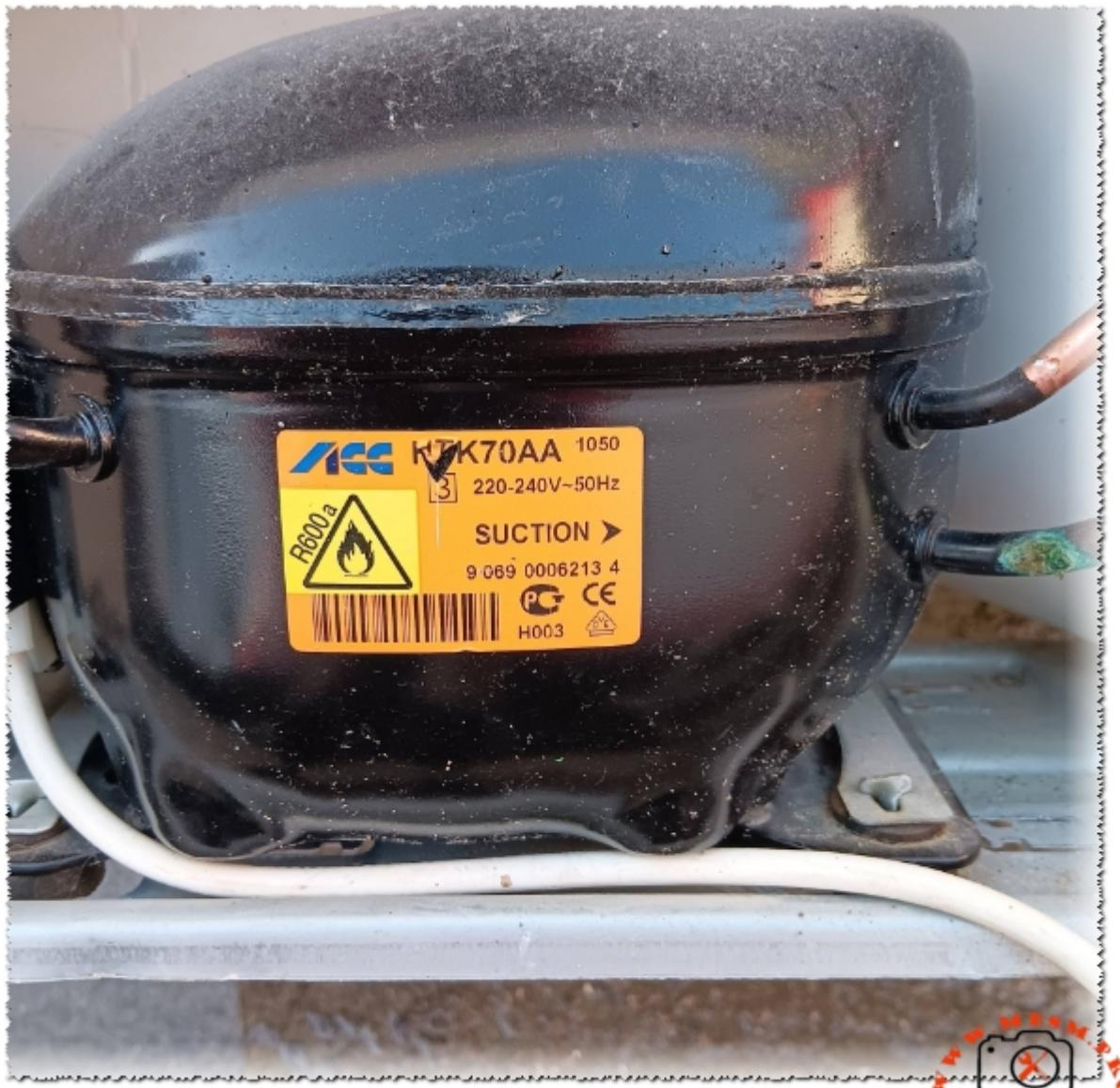
[mbsmpro.com-not recommended to replace compressor Jaxipera N1113Y with ACC HTK70AA](http://mbsmpro.com-not recommended to replace compressor Jaxipera N1113Y with ACC HTK70AA)
