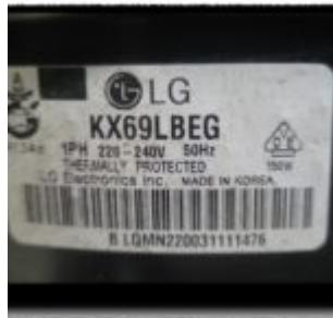
Mbsm.pro, Compressor, KX69LBEG, 1/5 hp, LG Electronics, R134a, 150 W, 1Ph, 220-240V 50Hz, LBP, Reciprocating, -35°C to -10°C, Refrigerator
