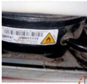
**Mbsmpro.com, Compressor, Jaxipera, VMH1111Y, 1/5 hp, Inverter, Cooling, R600a, 156 W, 22-75Hz, 1Ph 230V, LBP, Variable Speed, -35°C to -15°C**
