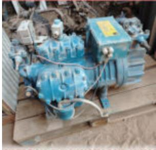
Frascold Z40-154Y is a semi-hermetic reciprocating compressor from Italy, rated at 40 horsepower for refrigeration applications with a displacement of 154 m<sup>3</sup>/h
