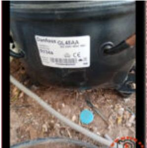
**Mbsmpro.com, Danfoss, GL45AA, 1/8 hp, LBP, Cooling, R134a, 81-96 W, 0.69-0.71 A, 1Ph 220-240V 50Hz, LBP, RSIR, -35°C to -10°C, Freezing**
