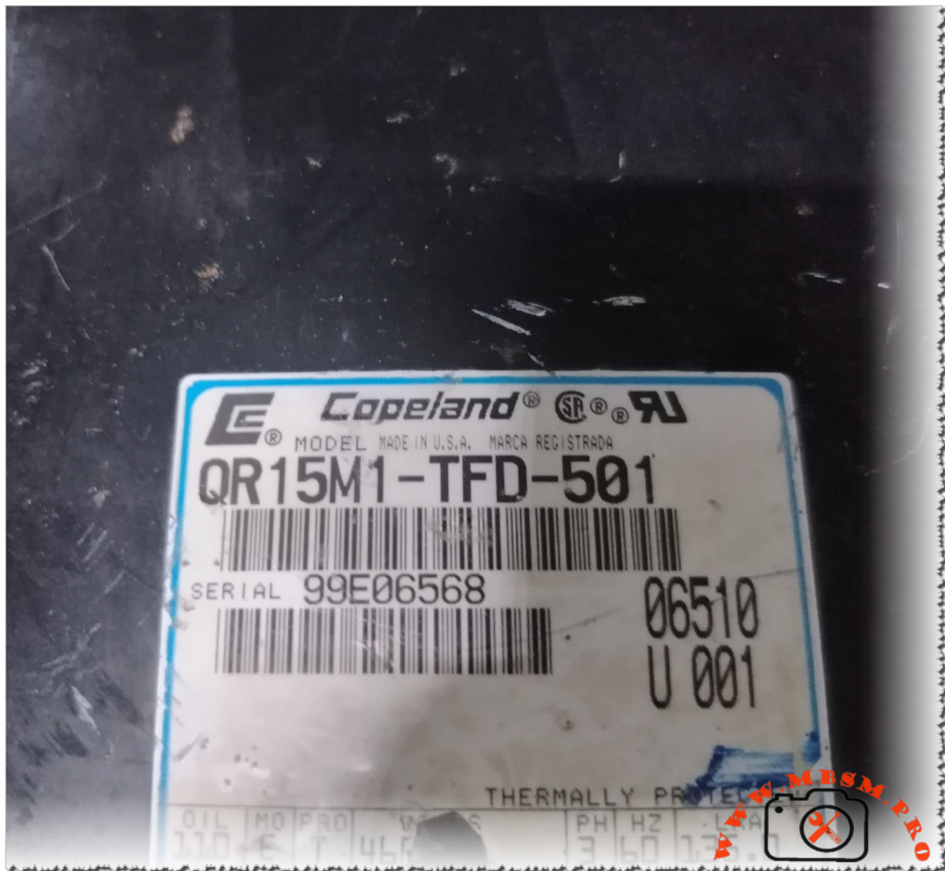
Copeland QR15M1-TFD-501 compressor mbsmpro copeland-hermetic-QR-2003Download
