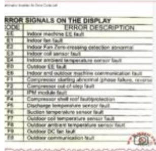
When your Kelvinator inverter split air conditioner displays an error code (E1, E2, E3, F1, F2, F3, etc.), it is signaling a specific system fault. This comprehensive guide explains every major error code—from sensor failures and communication breakdowns to compressor and power module protection triggers—and provides professional troubleshooting steps.
