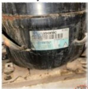
The Panasonic QB86C18GAX5 is a 1/4 HP reciprocating compressor engineered for high-efficiency Low Back Pressure (LBP) applications. Using R134a refrigerant and a displacement of 8.6cc, it delivers a cooling capacity of 201W. This guide provides technicians with essential technical data, including amperage, displacement, and a comprehensive cross-reference list for modern repairs.
