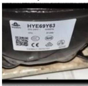
The Huayi HYE69Y63 is a highly efficient hermetic reciprocating compressor designed for low back pressure applications using R134a refrigerant. With a 1/5 HP rating and dual-frequency compatibility (50/60Hz), this motor is a cornerstone for domestic refrigerators and freezers. This comprehensive guide covers technical datasheets, electrical wiring, and professional replacement strategies for global cooling systems.
