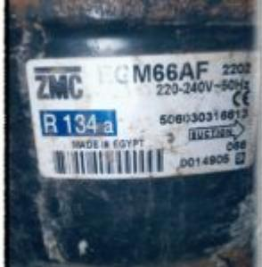
Yes, this compressor (**ZMC EGM66AF**) is an excellent fit for a **10-foot refrigerator**. It is rated at approximately **1/6 HP**, which is the industry standard for domestic fridges in the 10 to 12-foot range.
