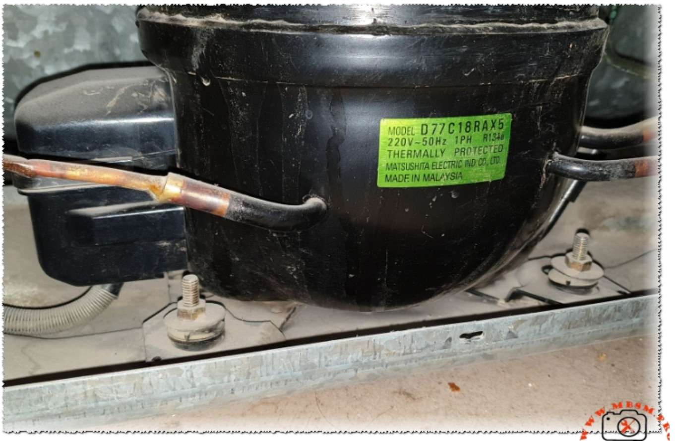
Compressor, Matsushita, D77C18RAX5, 1/4 hp, Panasonic mbsmpro mbsm.pro-Mbsmpro Compressor D77C18RAX5 RSIR 14 Hp D Series r134a LBP 186 W Toshiba Refrigerator 14 Feet GR-EFDownload
