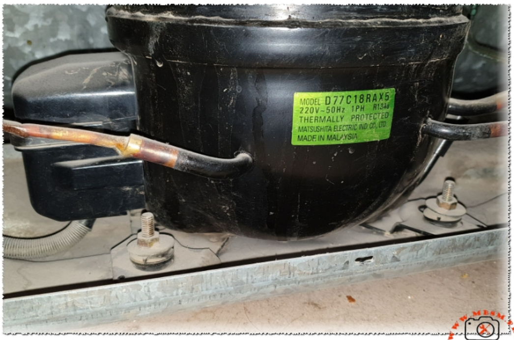
Compressor, Matsushita, D77C18RAX5, 1/4 hp, Panasonic mbsmpro
