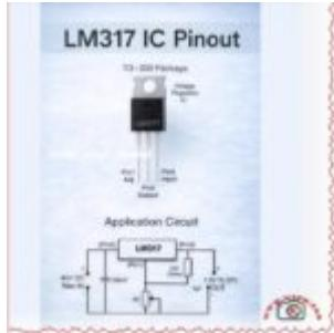
Mbsmpro.com, LM317 Voltage Regulator, TO-220, 1.2-37V, 40V IN, Pinout, Application Circuit, Thermal Design
