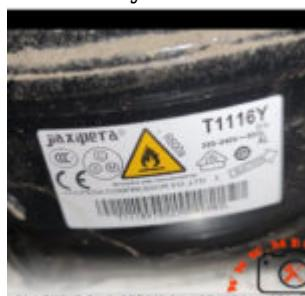
The Jaxpera T1116Y stands out as a reliable 1/5 HP hermetic piston compressor built for low back pressure (LBP) applications in mini fridges and small freezers. It runs on R600a refrigerant with a 10.5 cm<sup>3</sup> displacement, delivering 184W cooling capacity at -23.3°C.
