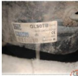
**Mbsmpro.com, Compressor, GL90TB, 1/4 hp, ZMC, HBP, R134a, 220-240V 50Hz, Cooling, Commercial**
