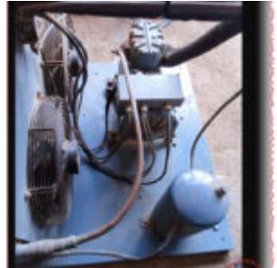
The photos show a Copeland condensing unit on a steel base, with a semi-hermetic compressor, air-cooled condenser and vertical liquid receiver designed for cold room applications. This type of refrigeration unit is widely used in commercial food storage because it delivers stable temperature control, good energy efficiency and straightforward maintenance for professional technicians.
