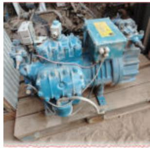
The photos capture a heavy-duty Frascold Z40-154Y semi-hermetic compressor, an Italian 40 HP unit designed for demanding freezer and cold-room applications. Its nameplate shows a displacement of about 154 m<sup>3</sup>/h and robust pressure ratings, while the blue cast-iron body and mounted controls reveal a machine built for long-term industrial refrigeration service.
