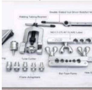
The NOCT-27545 ratchet wrench and NRVT35-275 flaring tool represent specialized HVAC instrumentation. This guide explains their functions, from creating perfect 45° flares to reaming tubing and driving fasteners in tight spaces, ensuring leak-free, professional installations.
