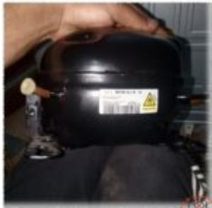
The Samsung MSV4A1A-L1B is a high-efficiency inverter compressor specifically engineered for R600a residential refrigeration systems. Operating between 54Hz and 216Hz, this 1/4 HP BLDC unit provides variable cooling capacity for premium side-by-side refrigerators. This professional guide covers essential technical specifications, diagnostic resistance checks, and critical installation protocols for modern refrigeration artisans.
