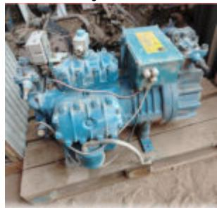
The photos capture a heavy-duty Frascold Z40-154Y semi-hermetic compressor, an Italian 40 HP unit designed for demanding freezer and cold-room applications. Its nameplate shows a displacement of about 154 m<sup>3</sup>/h and robust pressure ratings, while the blue cast-iron body and mounted controls reveal a machine built for long-term industrial refrigeration service.
