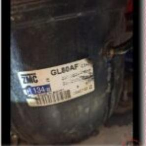
ZMC GL80AF R134a 1/5 HP hermetic refrigerator compressor technical data and applications
