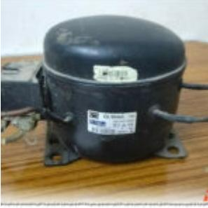
A 16 cubic feet Zanussi refrigerator typically relies on the GL90AA hermetic compressor, a compact piston unit built for R134a and low back pressure applications. This 1/4 HP motor offers cooling capacities from roughly 165 W up to around 346 W, giving enough reserve to maintain stable temperatures in family-size fridges even in hot kitchens.
