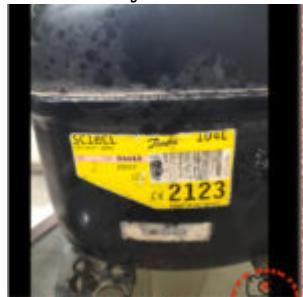
The Danfoss SC18CL compressor (104L2123) is a 5/8 HP hermetic reciprocating compressor designed for commercial refrigeration. Operating on R404A/R507 refrigerants at 220-240V 50Hz, it delivers 781W cooling capacity at -23°C for LBP/MBP applications. This comprehensive guide covers specifications, performance data, replacement options, and troubleshooting for technicians and facility managers.
