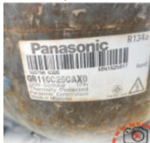
The Panasonic QB110C25CAX0 is a high-performance 1/3 HP reciprocating compressor designed for Low Back Pressure (LBP) applications. Operating on R134a refrigerant, it delivers 280W of cooling capacity at -23.3°C, making it ideal for large domestic freezers and commercial coolers. This guide provides technical data, COP efficiency tables, and compatible replacement models for technicians.
