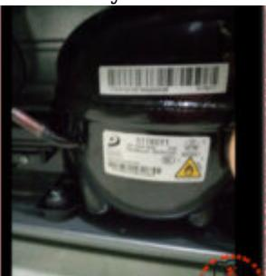
The Donper S118CY1 compressor is a cornerstone of modern domestic refrigeration, engineered for high efficiency in Low Back Pressure (LBP) environments. Utilizing R600a refrigerant, this 1/4 HP unit provides reliable cooling for large household refrigerators and freezers. This guide explores its technical parameters, electrical requirements, and the best cross-reference alternatives for field technicians.
