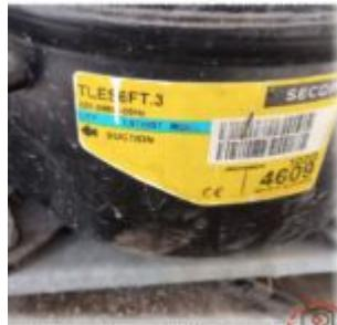
The Secop TLES6FT.3 is a high-efficiency hermetic reciprocating compressor designed specifically for Low Back Pressure (LBP) applications. Operating on R134a refrigerant, this 1/6 HP powerhouse is a staple in domestic refrigeration. This guide breaks down its technical performance, electrical characteristics, and provides reliable replacement options for field workers and engineers looking for precision.
