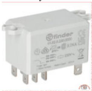
The Finder 66.82.8.230.0000 is a high-power, flange-mount relay designed for demanding switching tasks in HVAC, refrigeration and industrial control panels. With a 230 V AC coil and 30 A contact rating, it offers a compact but robust alternative to contactors in many applications, saving space while maintaining safety.
