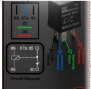
The MEISHUO S220 series relay, model MAA-S-124-C, is a 24-volt 5-pin SPDT automotive relay rated 20 A/10 A at 28 VDC. Its DIN 72552 terminal numbering—30, 85, 86, 87 and 87a—gives technicians a universal language for wiring and troubleshooting in vehicles, HVAC equipment and industrial control panels.
