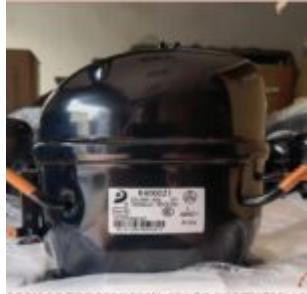
The Donper K400CZ1 is a hermetic reciprocating compressor designed for commercial refrigerators and chest freezers operating with refrigerant R134a on 220-240V 50Hz single-phase power. It offers roughly 1/2 hp class performance with about 400 W cooling capacity, making it suitable for medium-size display cabinets and storage equipment in supermarkets and restaurants.
