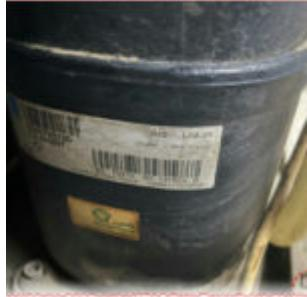
The Tecumseh / L'Unité Hermetique CAJ9480T is a 5/8 HP hermetic compressor delivering about 1 968 W of cooling capacity for R22 commercial refrigeration systems. It is widely used in small cold rooms, display cabinets and compact condensing units. This Mbsmgroup guide explains its main specifications, applications, installation tips and key technical PDFs.
