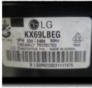
The LG KX69LBEG is a high-performance 1/5 HP reciprocating compressor designed for Low Back Pressure (LBP) domestic refrigeration. Operating on R134a refrigerant at 220-240V/50Hz, this thermally protected unit is the standard for LG's cooling reliability. In this guide, we break down its displacement, amperage, and provide a comprehensive list of equivalent replacement models.
