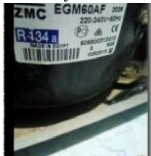
The ZMC EGM60AF is a high-performance hermetic compressor designed for low back pressure applications in domestic refrigeration. Engineered with precision in Egypt, this 1/6 HP unit operates on R134a refrigerant and is tailored for 220-240V 50Hz power systems. It offers a reliable cooling solution for small to medium household refrigerators and upright freezers worldwide.
