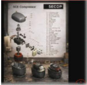
Understanding the inner workings of a Secop SCE hermetic compressor is essential for any refrigeration technician or engineer. This comprehensive guide breaks down the complex internal components—from the crankshaft to the valve plate—providing a detailed exploded view. Whether you are troubleshooting or studying mechanical design, our professional analysis offers the clarity needed for modern cooling systems.
