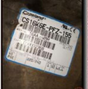
The Copeland CS16K6E-PFZ-155 is a high-efficiency hermetic reciprocating compressor designed for commercial refrigeration. Operating at 220-240V and 50Hz, this 1.25 HP powerhouse is optimized for R404A and R507 refrigerants. Known for its durability in medium-temperature applications, it features POE oil and thermal protection, making it a reliable choice for cold rooms and professional cooling systems.
