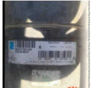
On the faded nameplate of this weathered compressor shell, one line stands out with absolute clarity: CAJ9480T - R22/R502 - Made in France. It is the unmistakable signature of a Tecumseh L'Unité Hermétique fully hermetic compressor, a workhorse still beating quietly inside countless small cold rooms and refrigerated cabinets in everyday commercial settings.
