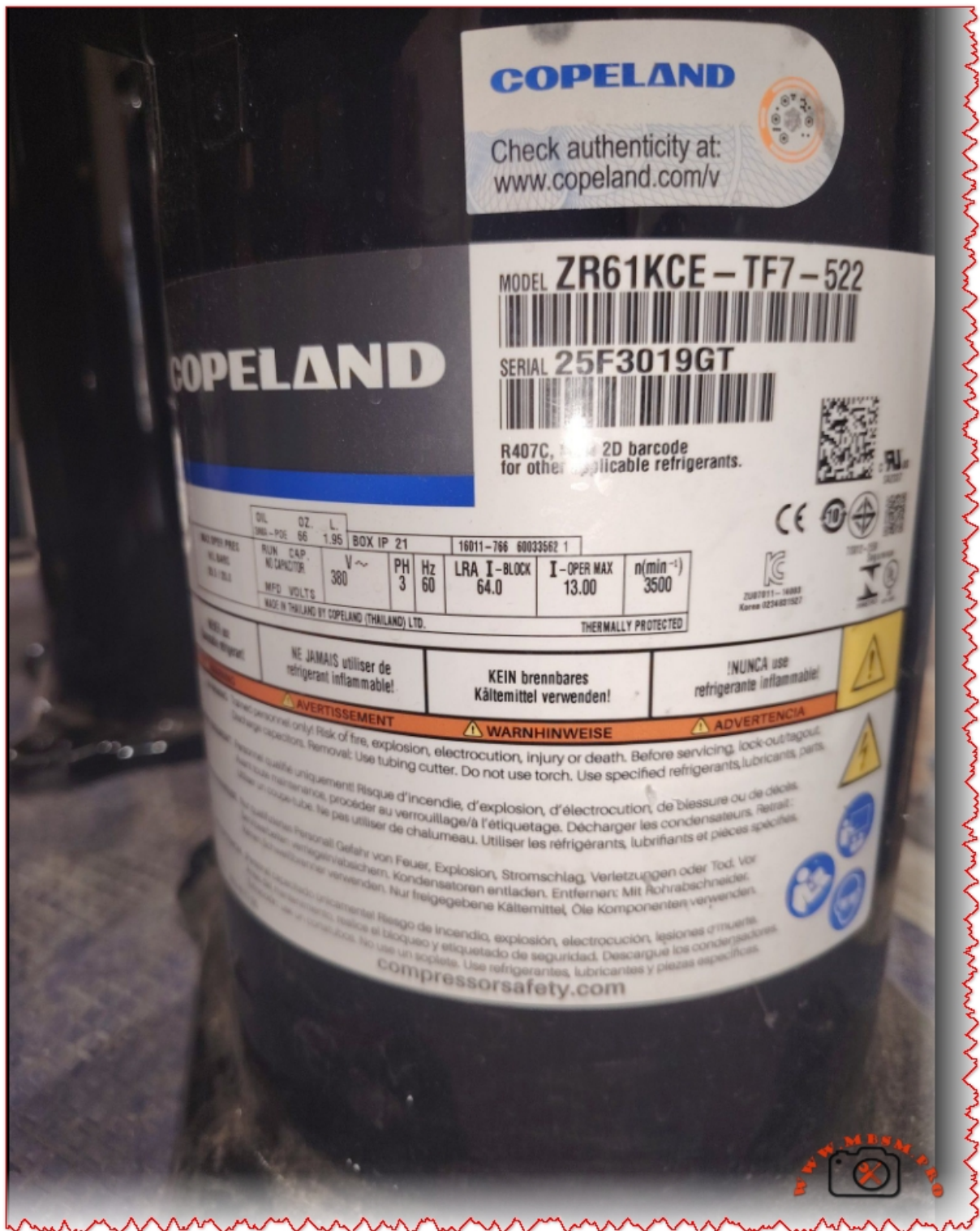
Mbsmpro.com, Copeland, ZR61KCE-TF7-522, 5 hp, Scroll Compressor, Air Conditioning, R407C, 3Ph 380-420V 50Hz, HBP, Original or Fake, Authenticity Guide
