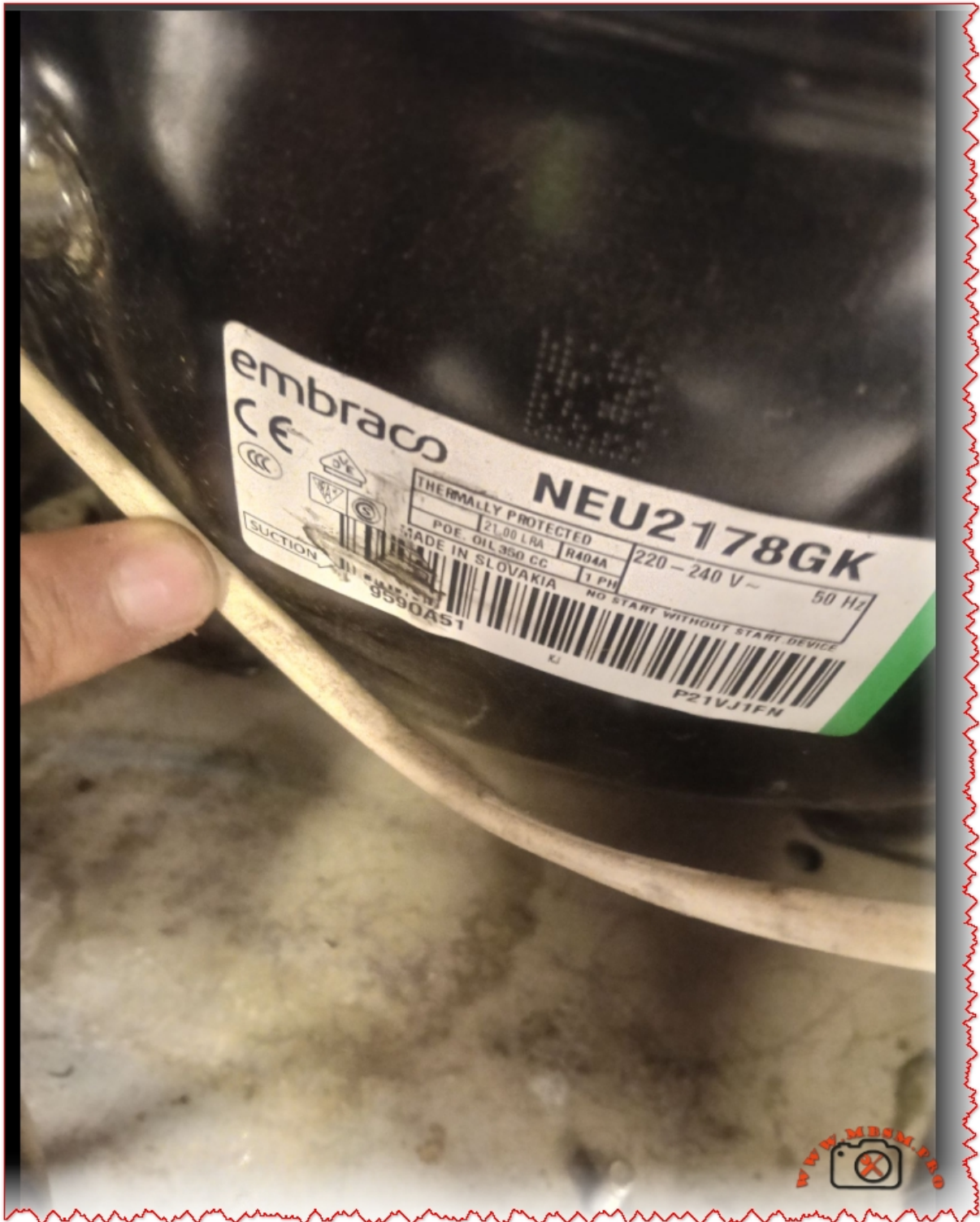
Mbsmpro.com, Embraco, NEU2178GK, 1 HP, LBP, R404A, 220-240V, 50Hz, 16.8 cc, CSR, Commercial Freezer Compressor
