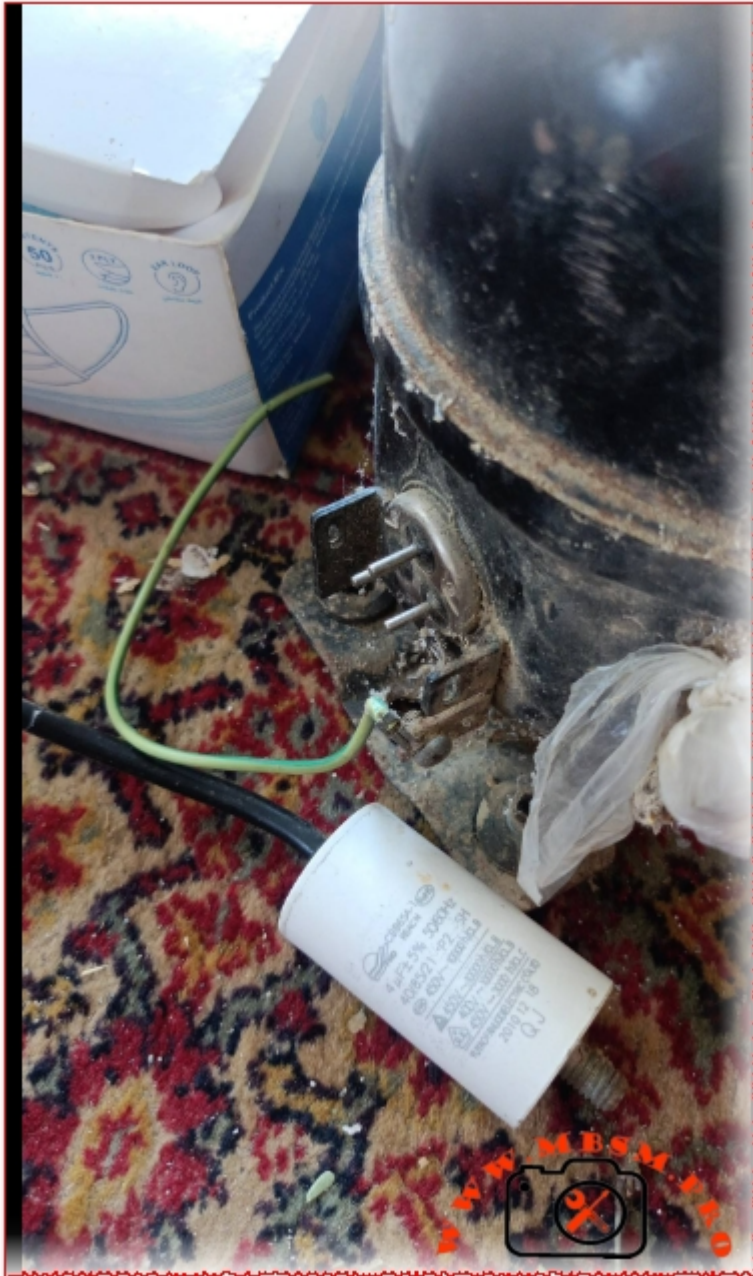
WS57H Compressor, 1/6 hp, Capacitor Requirement 4mf mbsmpro
