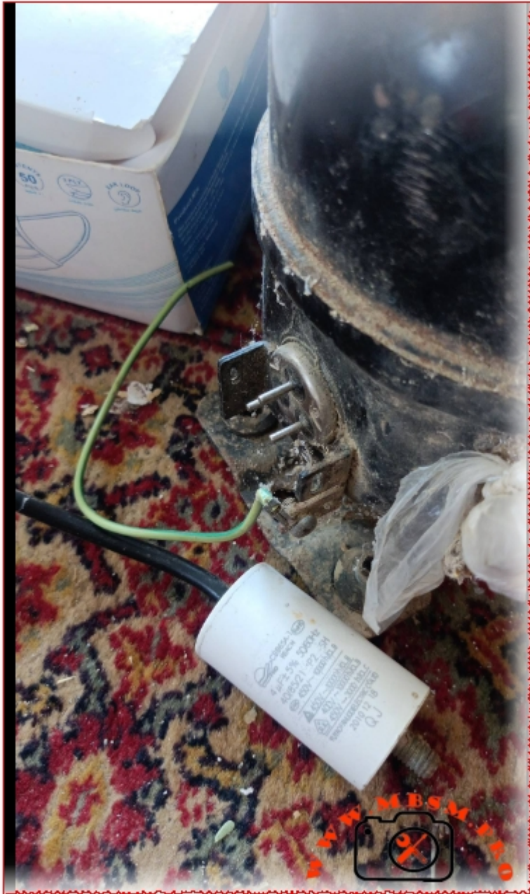
WS57H Compressor, 1/6 hp, Capacitor Requirement 4mf mbsmpro
