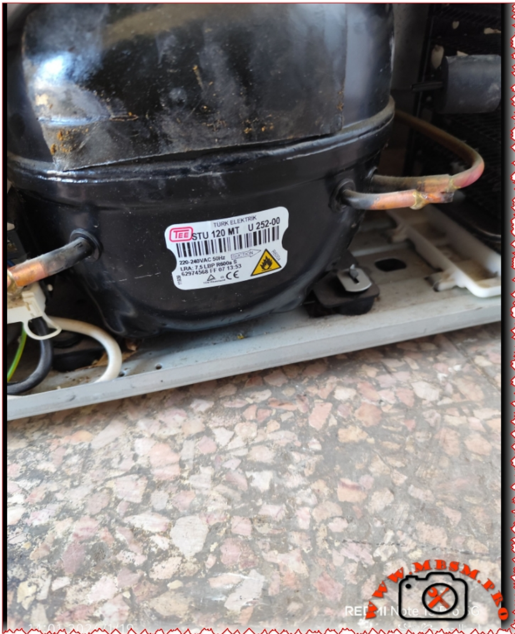
Compressor, STU 120 MT, 1/6 hp mbsmpro
