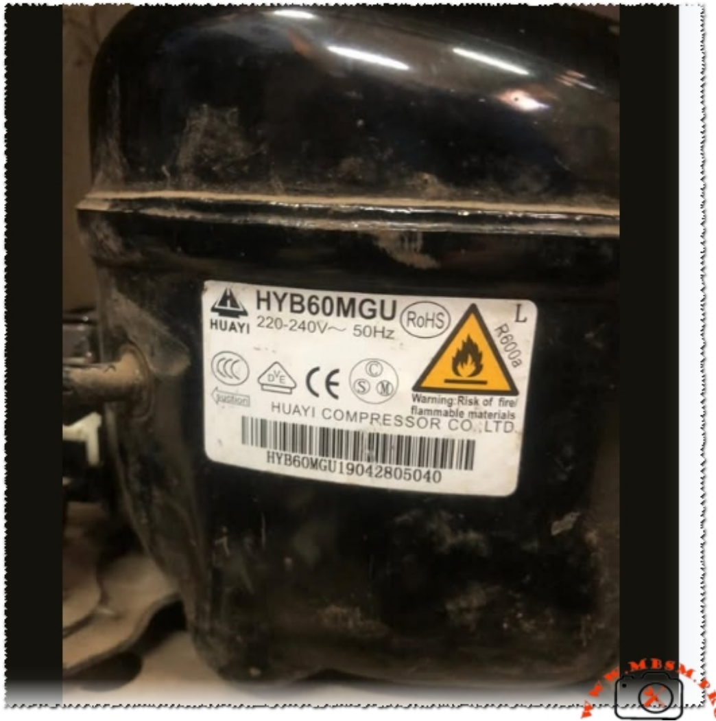
Huayi HYB60MGU Compressor 1/7 HP R600a LBP mbsmpro
