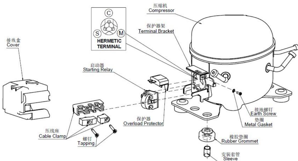
Note: Each of the starting relay and thermal protector、cover and the screw assembly is separately provided by our company.
